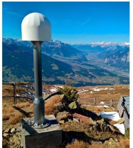
Fig. 4: The APOS reference station PAT2 at Patscherkofel (H = 2298 m, ellipsoidal height – ETRS89)
