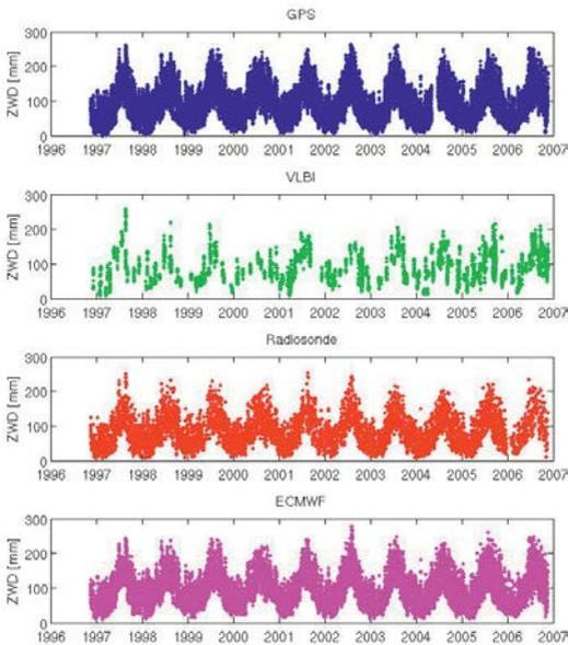
Fig. 4: Time series of ZWD estimated from various instruments at the Onsala Space Observatory, Sweden: GPS, VLBI, radiosondes, and ECMWF data.
