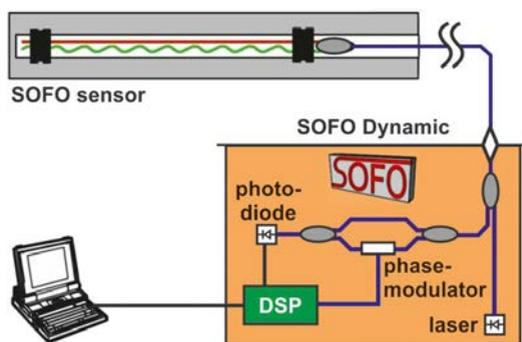
Fig. 1: Schema of the SOFO Dynamic system using a Mach-Zehnder interferometer and a DSP (digital signal processor) unit, after [10]
