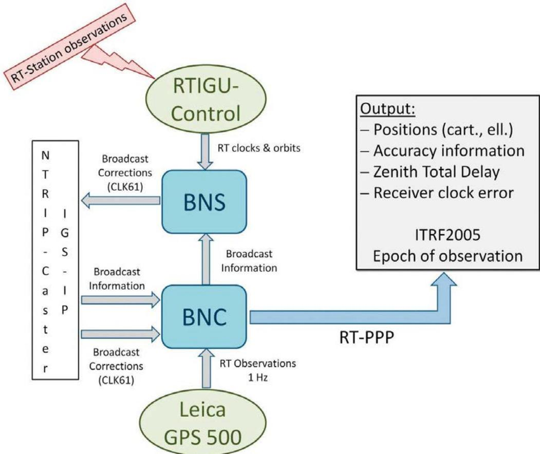
Fig. 3: Processing scheme of the RT-PPP experiment
