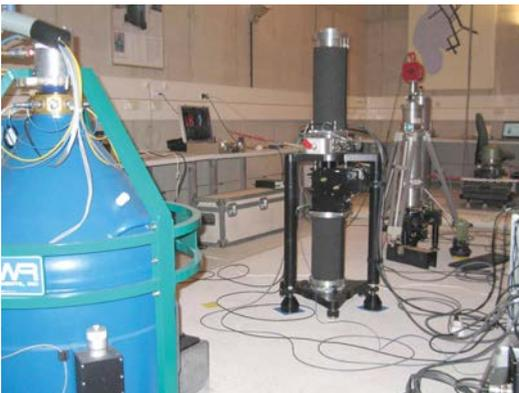
Fig. 5: Comparison of three types of gravimeters (GWR, FG5, JILAg) in the gravity laboratory at the Conrad Observatory Trafflberg of ZAMG
