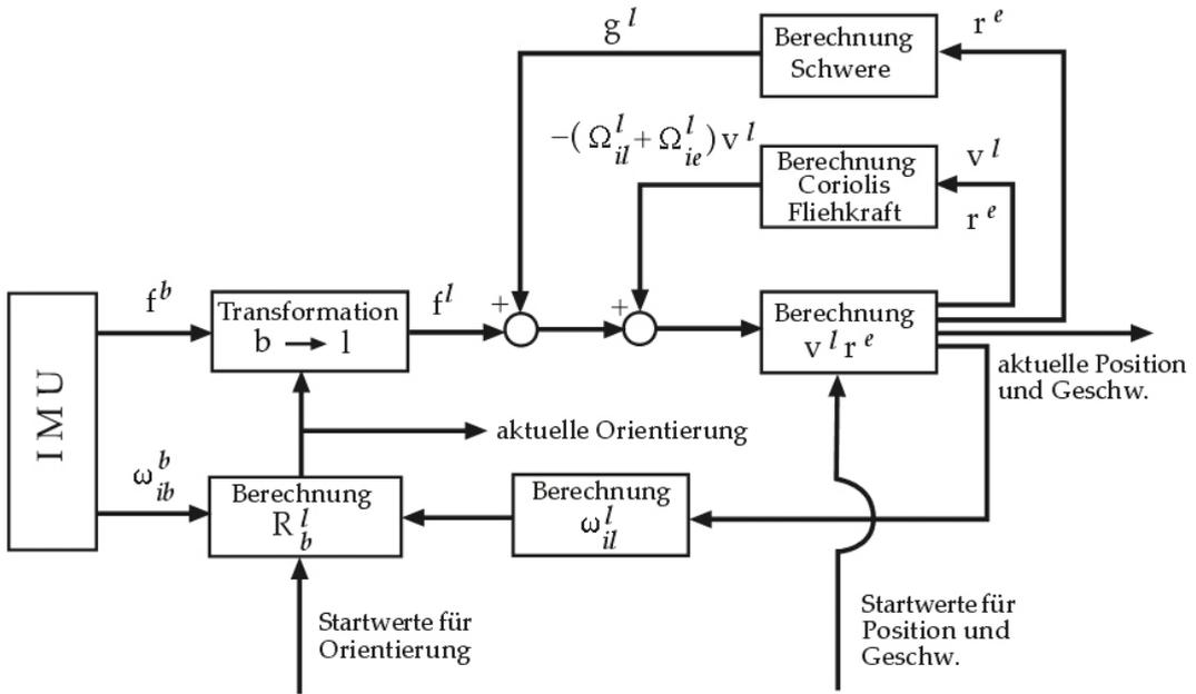
Fig. 1: Procedure for solving the navigation equations
