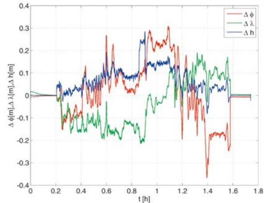
Fig. 2: Deviations between new Kalman-filter and Waypoint trajectory
