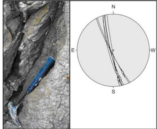
*Fig. 4: Structural geologic field measurements of the faults shown in Fig. 3 indicate a NNW-SSE orientation. The field measurements were plotted using Schmidt's net plots. It is important to note that many linear features in the host rock surrounding the mass movement have similar orientation.*
