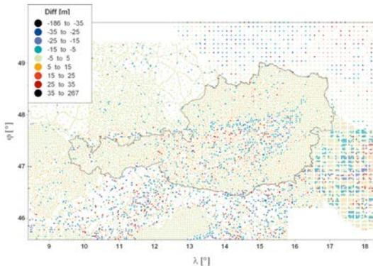
Fig. 4: Differences between the station heights of the gravity observation points and the newly established height model used for GEOAUT.
