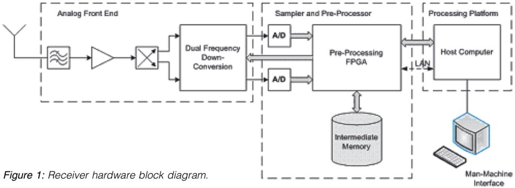
Figure 1: Receiver hardware block diagram.
