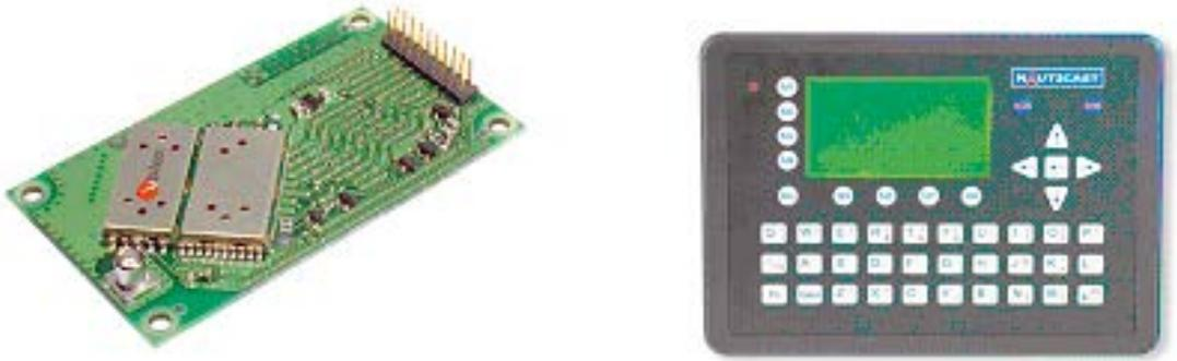
Figure 3: EMAG functional demonstrator overview (left: u-blox GPS/EGNOS receiver module; right: NAUTICAST AIS transponder).
