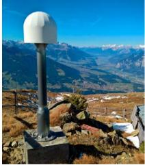
**Fig. 4:** The APOS reference station PAT2 at Patscherkofel (H= 2298 m, ellipsoidal height – ETRS89)
