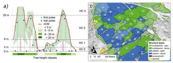
Fig. 2: (a) Classification of laser echoes into height classes according to nCM height; (b) derived structure type classification of forest sample area. [41]
