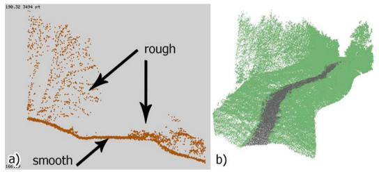
Fig. 3: (a) Profile of forest road (smooth surface) with roadside vegetation and overhanging trees (rough surface); (b) result of 3D segmentation of a forest road, black dots represent the road. [55]
