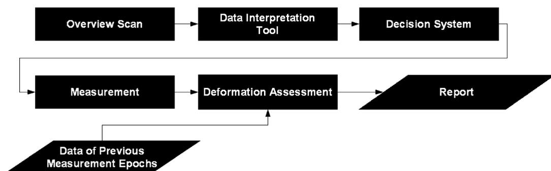
Figure 3: Abstract, simplified measurement and analysis procedure.
