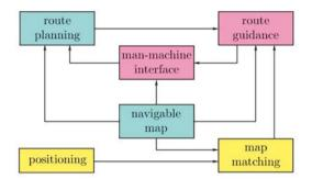
*Figure 1:* Components of a pedestrian navigation system.
