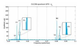
Figure 2b: CLEAN spectrum of the diurnal and subdiurnal tidal frequency bands from GPS-derived  $y_p$  time series
