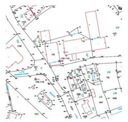
Figure 4: Example of a digital cadastre map (DKM) used for fixing the horizontal position of the gravity stations.
