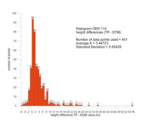
Figure 2: Histogram of the differences between the elevations of geodetic benchmarks (TP) and their corresponding interpolated DTM heights within a mountainous area (Austrian map sheet 119).
