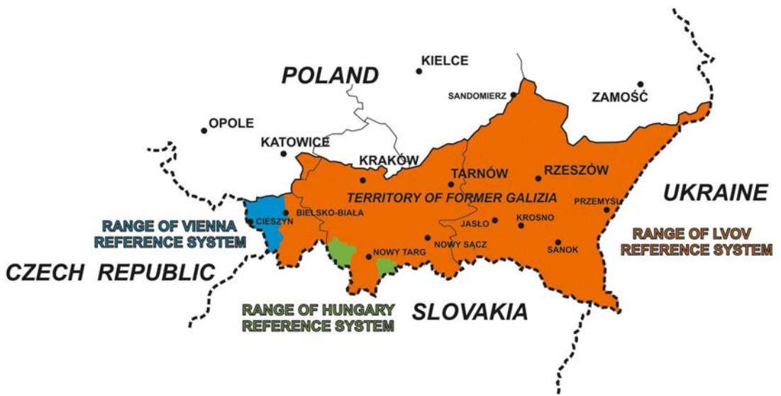
Fig. 1: Coverage of the former Austrian cadastre in Poland and the respective reference systems used for cadastral surveys (source: [3] modified by the authors)
