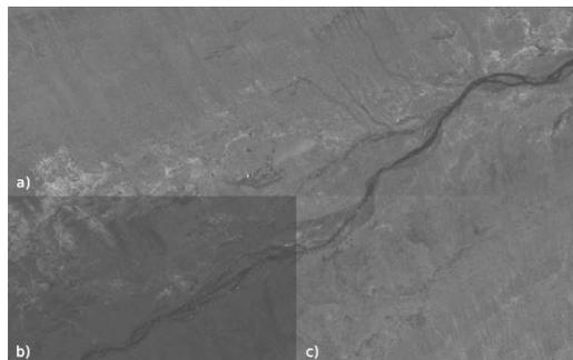
**Fig. 3:** Corrected vs. radiometric adjusted amplitude values: a) corrected amplitudes (October 11, 2007, H07); b) corrected amplitudes (October 5, 2004, H04); c) corrected and radiometric adjusted (the radiometric adjustment factor is 1.74; October 5, 2004, H04); the graphic shows amplitude images (range from 0, black to 160, white)
