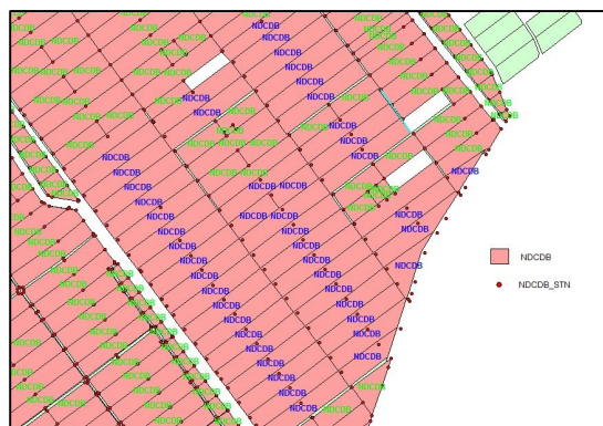
Figure 4: Content of NDCDB block representing coordinate values for cadastral markers and their respective parcels as shown in Figure 4
